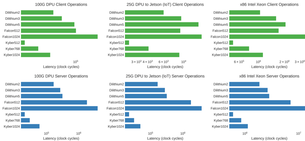
Figure 2-4: Average latency results in CPU clock cycles introduced by the execution of PQC cryptography. The first row shows the latency the client machine is penalized with. The second row represents the tax in CPU cycles introduced by PQC operations when performed on the server machine
