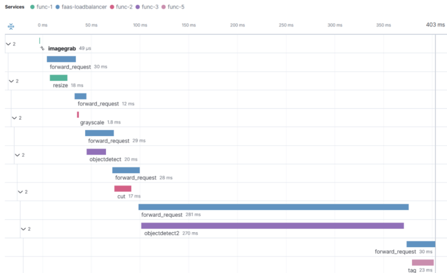
Figure 5-5: Sample visualization of the function execution and invocation latencies in the serverless test scenario.
